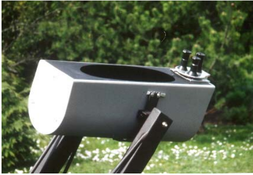
Herrig TCT Telescope (This telescope can be made of two spherical mirrors)
